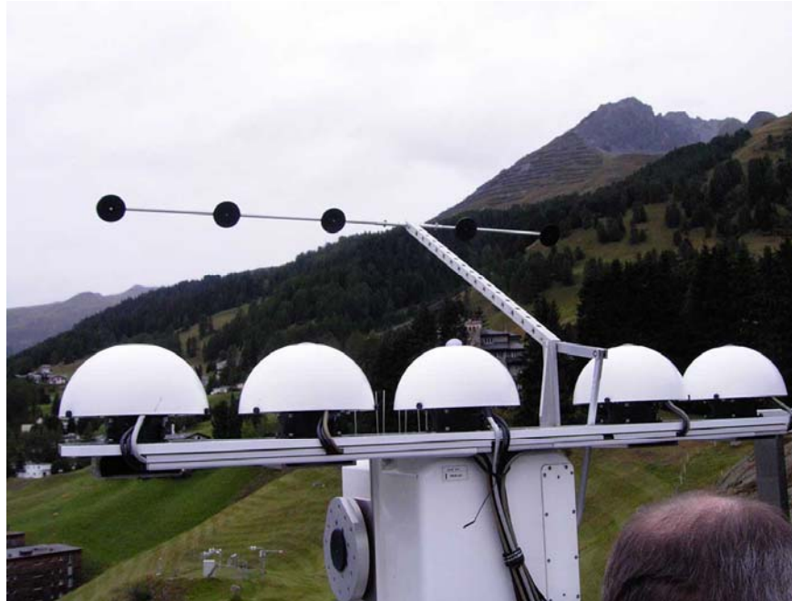
世界赤外放射計準器群(WISG: World Infrared Standard Group of pyrgeometers)
