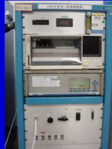
Total hydrocarbon analyzer
