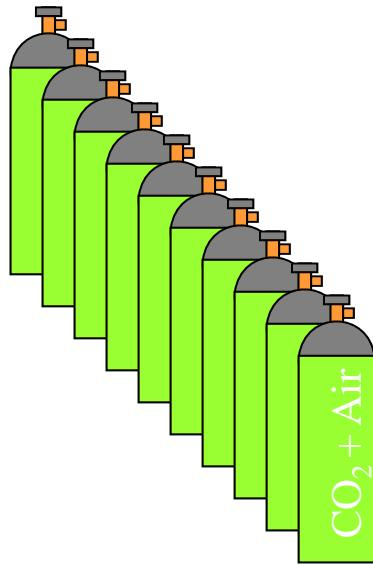
10 of gravimetric one-step dilution cylinders
